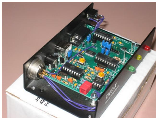
*Figure 1 – An interior view of TNC-X, one of many available KISS mode TNCs. Photo from the manufacturer’s Web site.*
